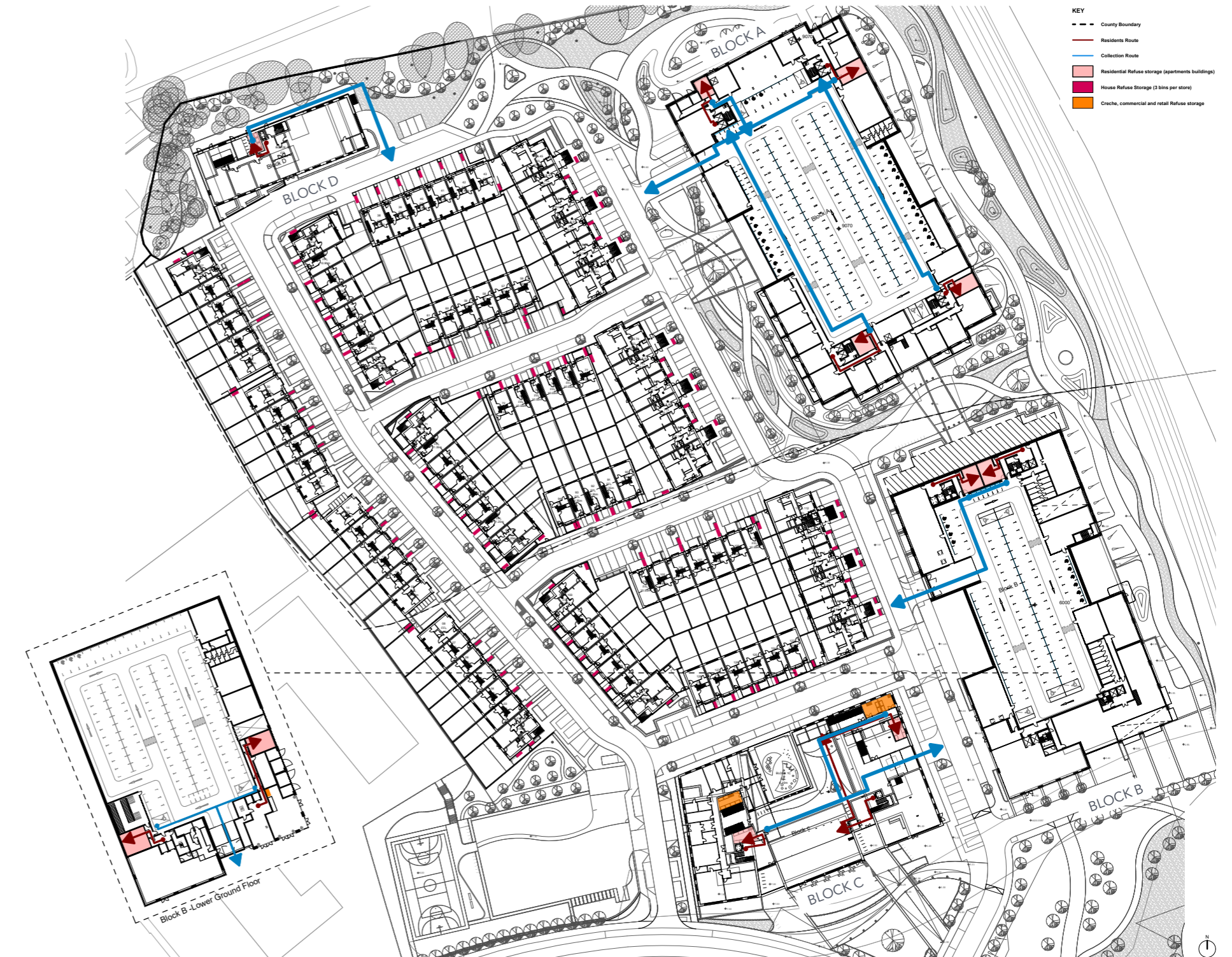
Fig.43 Ground Floor Plan showing refuse storage/collection routes
