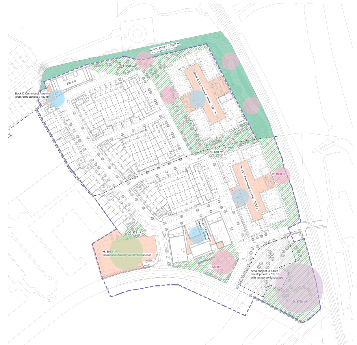
Fig.44 Public Open Space, residents external communal space and childrens play area diagrams
