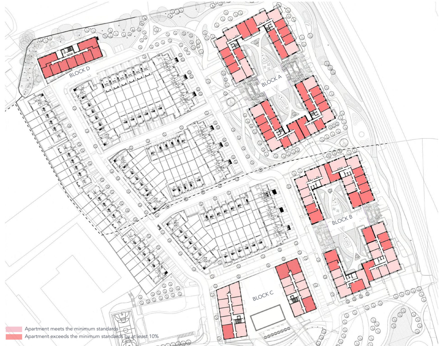
Fig.9 10% Oversized Apartment Diagram for typical floors on apartment buildings
