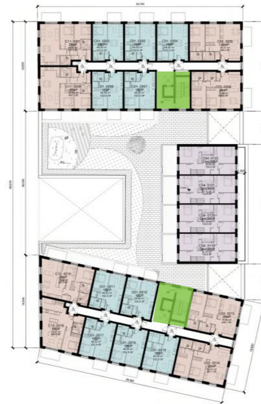
Fig.28 Block C Typical Floor - 9 Units per core
